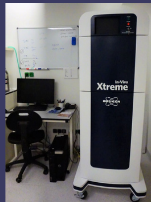
Optical Imager • Fluorescence • Luminiscence • Reflectance • Cherenkov radiation
