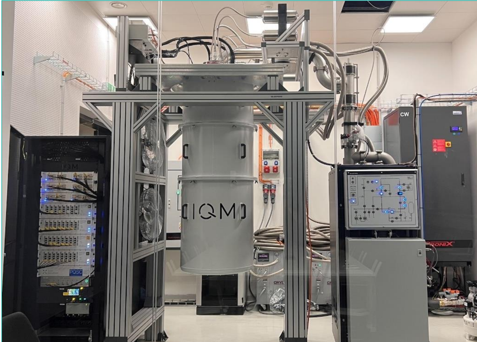
Superconducting technology, 24 qubits in a star-shaped topology
