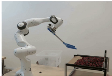
Output: tool manipulation skill transferred to a robot
